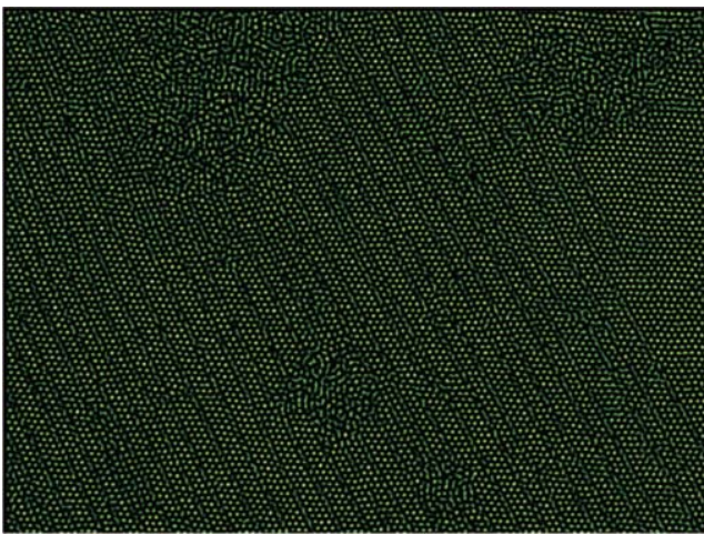
FIG. 12. (Color online) Lakes in the eight-layer buckled crystalline film. The parallel stripes reflect the buckling. The upper left corner without stripes is normal crystal. The buckling remains in the solid/liquid coexistence regime. Again, images are 2D slices from the middle of the film. Liquid regions look about the same in all layers.
