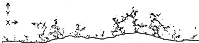
FIG. 1. Experimental image of a deposit of ellipsoids (major-minor aspect ratio \varepsilon = 2.5 ). The contact line is highlighted. x and y directions are indicated.
