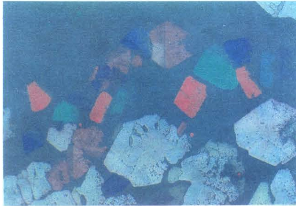
FIG. 2. Surface crystallites as viewed under an optical microscope.
