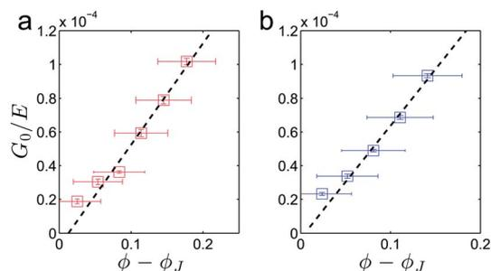
Fig. 6 Dimensionless static shear modulus,  $G_0/E$  vs.  $|\phi - \phi_J|$  for aqueous suspensions of (a) monodisperse and (b) bidisperse PNIPAM particles. The error bars for  $\phi - \phi_J$  are derived for uncertainty of  $\phi_c = 0.58$ – $0.64$ . Dashed lines are best linear fits expected for Hertzian particles ( $\alpha = 5/2$ ).
