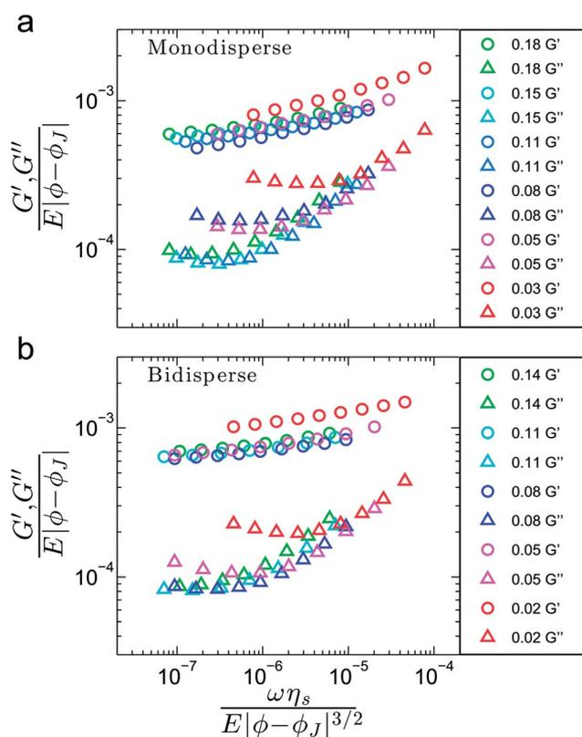
Fig. 7 Volume-fraction-difference-scaled dimensionless moduli,  $G'/E$  and  $G''/E$ , as function of dimensionless oscillatory frequency,  $\omega\eta_s/E$  for (a) monodisperse and (b) bidisperse PNIPAM microgel spheres at  $\phi - \phi_J > 0$ , assuming Hertzian interactions.
