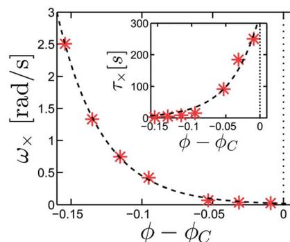
Fig. 8  $G'$  and  $G''$  cross-over frequency,  $\omega$  as a function of  $\phi - \phi_c$  at  $\phi - \phi_c < 0$ . Inset: corresponding time scale,  $\tau$ , versus  $\phi - \phi_c$ . Dashed lines indicate exponential fits.
