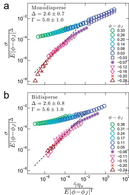
Fig. 3  $\sigma$  vs.  $\dot{\gamma}$  for aqueous suspensions of (a) monodisperse and (b) bidisperse PNIPAM microgel spheres scaled with  $|\phi - \phi_c|^\Delta$  and  $|\phi - \phi_c|^\Gamma$ , respectively. Best-fit values of  $\Delta$  and  $\Gamma$  are given inside the figures. The dashed lines indicate slopes of unity.
