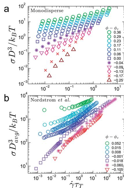
Fig. 4 Rescaled stress/strain-rate data sets reproduced from (a) Fig. 2a and (b) Nordstrom *et al.* (Fig. 3),<sup>1</sup> respectively. Stress is rescaled by the thermal stress scale ( $D^3/k_B T$ ), and strain-rate is rescaled using the thermal time scale ( $\tau_T$ ) as described in the main text.
