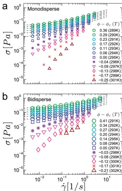
Fig. 2 Stress ( $\sigma$ ) vs. strain rate ( $\dot{\gamma}$ ) data for aqueous suspensions of (a) monodisperse and (b) bidisperse PNIPAM microgel spheres, obtained using bulk rheology. Each curve is obtained at a different temperature corresponding to a different volume fraction,  $\phi - \phi_c$ . Dashed lines are Herschel–Bulkley best-fits to the data in the solid regime.
