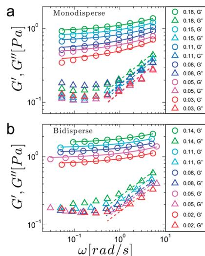
Fig. 5  $G'$  and  $G''$  as function of  $\omega$ , for aqueous suspensions of (a) monodisperse and (b) bidisperse PNIPAM microgel spheres. Data are obtained applying a maximum strain amplitude of  $\gamma = 0.01$ .  $\phi - \phi_J$  corresponds to temperature steps of 0.5 K (*cf.* Fig. 1). The data are fit to  $G' = G_0(1 + \sqrt{\omega/(2\omega_n)})$  (solid lines), and  $G'' = G_0(\sqrt{\omega/(2\omega_n)})$  (dashed lines), where  $G_0$ , and  $\omega_n$  are fitting parameters.
