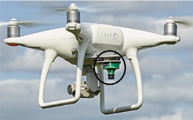
Figure 3. Sentera Multispectral Sensor Upgrade for DJI Phantom 4.
