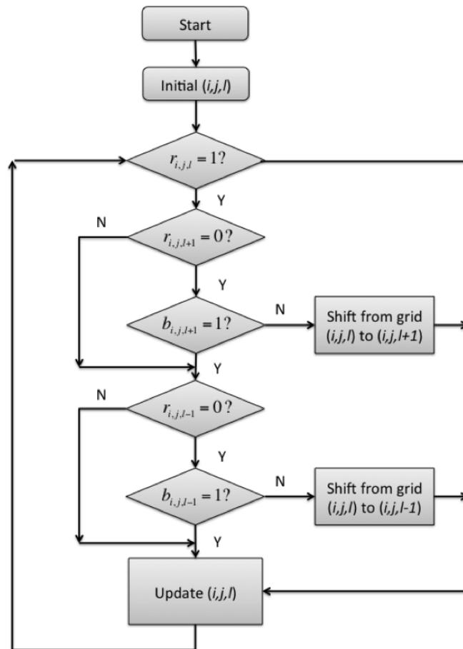
Figure 4. Flow chart of the grid shifting with sector capacity constraint.
