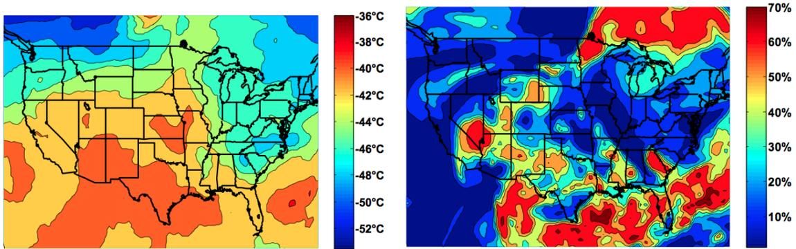
Figure 1. Contours of temperature and RHw at 34,057 feet at 8AM EDT on August 1, 2007.
