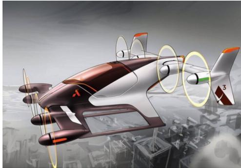
**Fig. 1** Airbus Vahana with tandem tilt-wing configuration during the cruise phase [17].
