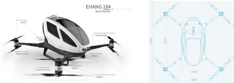
Fig. 1 EHang 184 specs and configuration [12].
