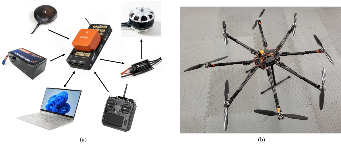
Fig. 7 (a) Schematic diagram of the electrical components of the octocopter. The Cube Orange (ADS-B Carrier Board) flight controller ( center ) is connected to all components as the main hub. The lipo battery ( center-left ) provides the power to run all components. The electronic speed controller ( center-right ) receives the control inputs from the Cube to regulate the brushless motor ( top-right ) speed. The GPS module ( top-left ) sends the position information signals to the Cube; then, it transfers the information to GCS. ( bottom-left ). The RC controller ( bottom-right ) will be used in the emergency situation to manually control the octocopter. (b) Tarot T18 octocopter, built to validate our proposed controllers.
