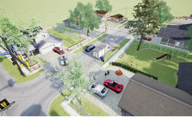
Fig. 5. Simulated suburban environment for a UAS package delivery scenario. The scene integrates 3D assets reconstructed via the SAM3D pipeline (e.g., residential house, vehicles, and school bus) with supplemental high-fidelity assets from the Epic Games ecosystem. Moving actors were placed in the environment with pre-defined spline paths to simulate a dynamic suburban package delivery landing scenario. This hybrid environment serves as the high-fidelity testbed for synthetic data collection and automated ground-truth annotation procedures.
