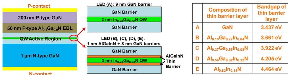
Fig. 2. Schematics of InGaN QW LEDs consisting of 3 nm  $\text{In}_{0.28}\text{Ga}_{0.72}\text{N}$  QW with conventional 9 nm GaN barriers [LED (A)] and novel barrier design of 1 nm thin large-bandgap AlGaInN barrier together with 8 nm GaN thick barrier. The inserted table summarizes the material compositions and bandgaps of the thin lattice-matched AlGaInN barriers used in the study.
