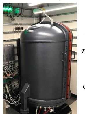
Our crystal growth facility is unique in the world due to our ability to pursue ammonothermal single crystal growth in novel, extremely corrosion resistant Mo-alloy, in traditional NiCr superalloy (right) or in SS autoclaves.
