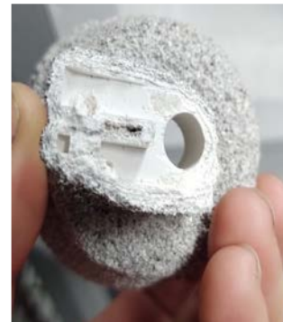
Ceramic shell after burnout
