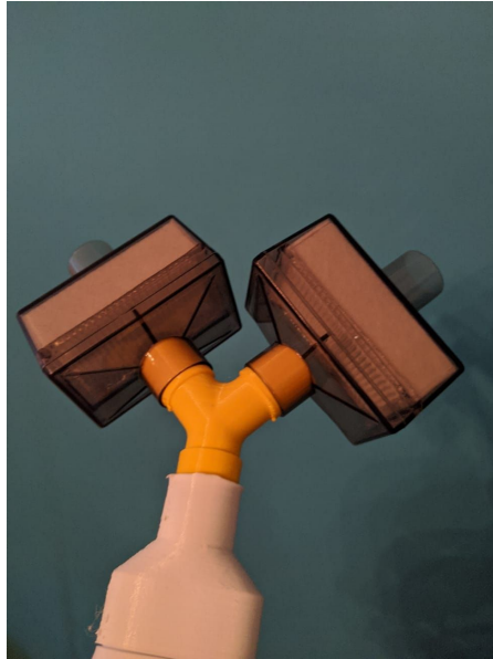
Printing snorkeling mask adapters for air filters
