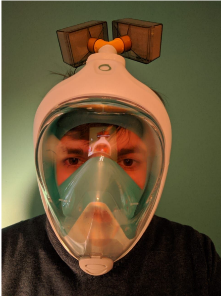
Printing snorkeling mask adapters for air filters
