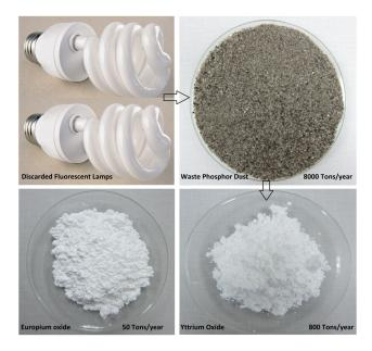
8,000 tons of phosphor dust waste are generated each year in the United States from disposed fluorescent lamps. This waste phosphor dust can contain a resource of up to 800 tons/year of yttrium oxide and 50 tons/year of europium oxide.
