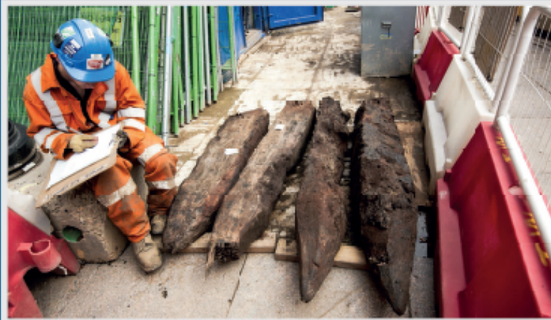
Elm timber piles from the 16th century cemetery wall foundation at Bedlam Burial Ground being recorded
