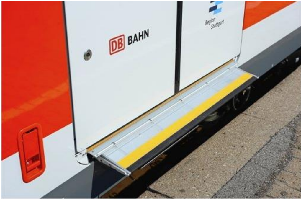
Figure 29. Mechanical Gap Fillers on a German Train
