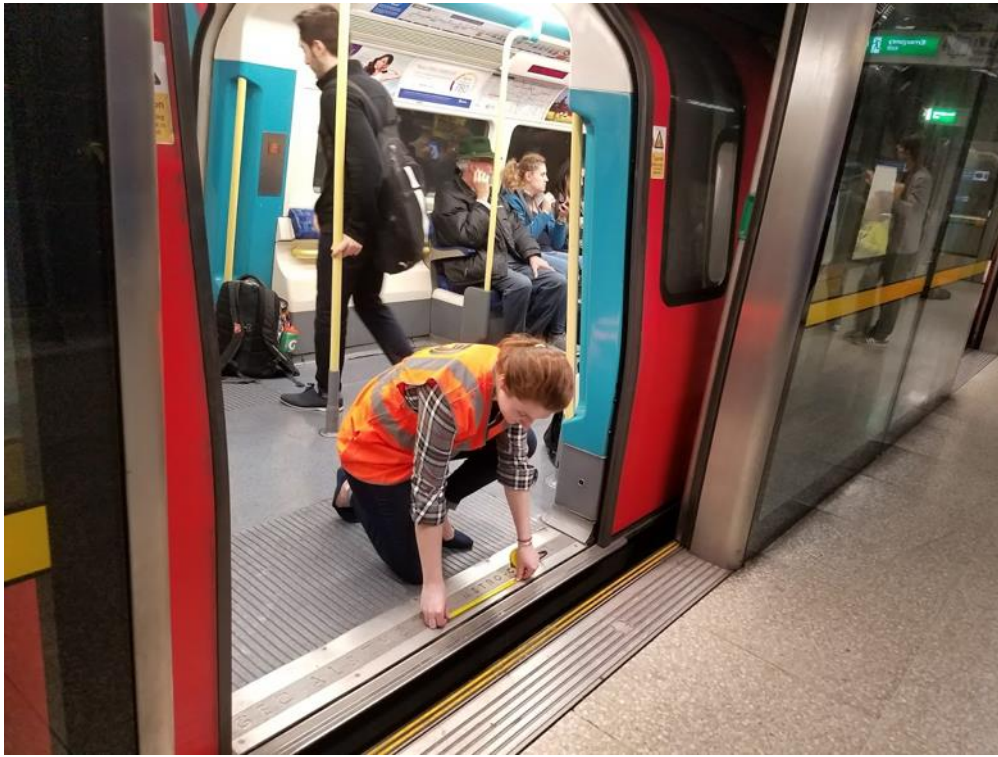
Figure 14. Performing a manual measurement of the stopping accuracy, second method
