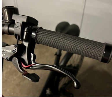
Left handlebar and parking lock system.
