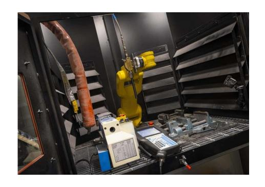
VRC Gen III **Cold Spray System** - Capable of producing coatings with diverse compositions on a multitude of substrates
