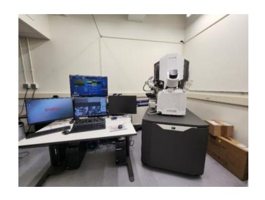
Thermo Scientific Scios 2 DualBeam – Focused Ion Beam Scanning (FIB-SEM) Equipped ETD, in-lens trinity detection system, Ivd, ICE detector, retractable DBS detector, retractable STEM detector, Oxford Instruments Ultim Max 100 mm2 EDS and Symmetry 2 EBSD system
