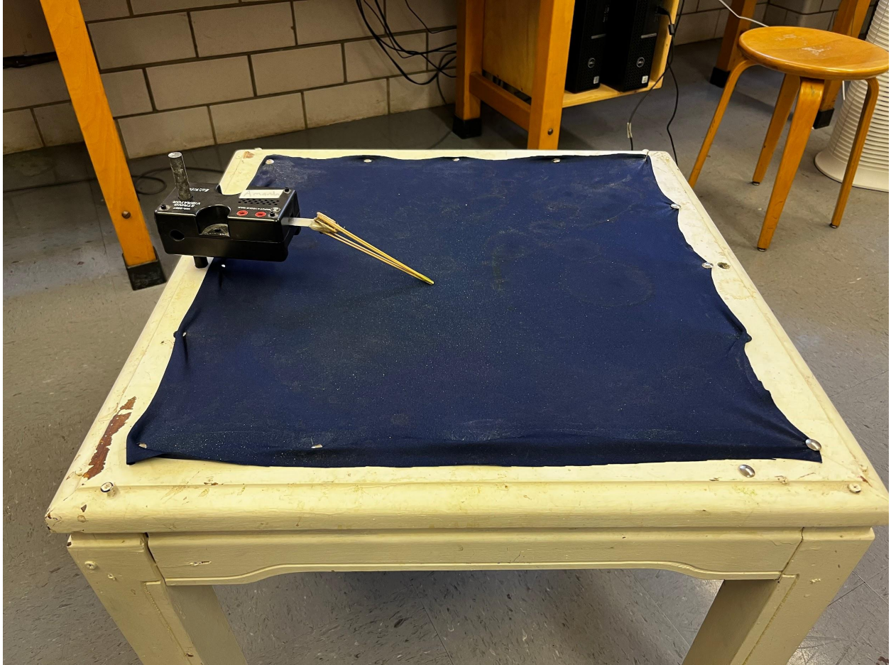
Figure 6: A table with a soft, flexible material spread across it. Ontop of the dark blue fabric is an oscillator with a point that when connected up causes oscillations. This is also called a "chladni plate". You would add sand or some other small particle material on top (styrofoam?)
