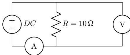
Figure 3: This is an example circuit diagram. On the left we have the DC power supply input. In the middle is the lightbulb. On the right is the voltmeter, which is parallel to the lightbulb. Then on the bottom of the circuit is the ammeter, which is in series with the lightbulb and DC power supply.
