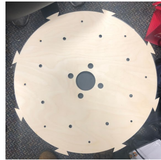
Figure 15. Wooden plate that holds the funnels.
