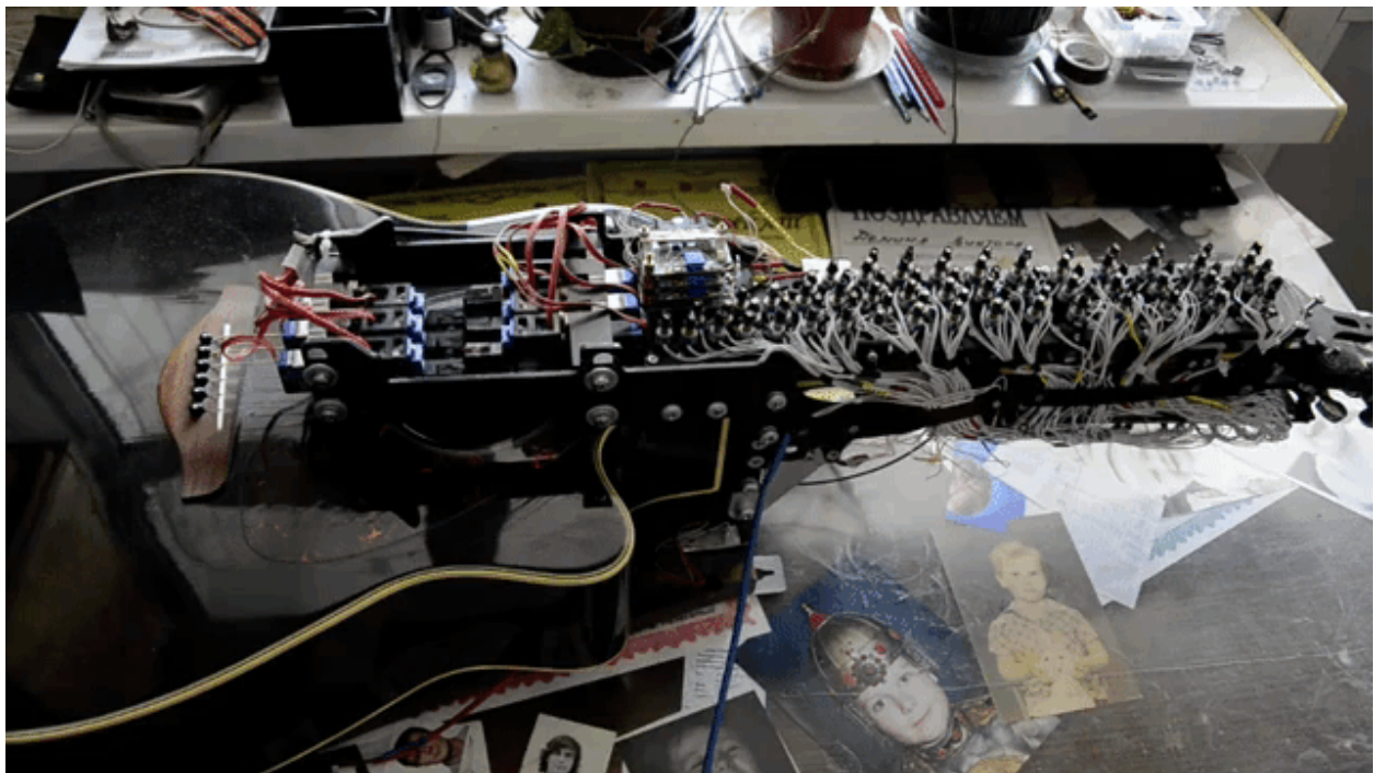
Figure 1: Vladimir Denin's guitar robot. Note the fretboard blanketed in solenoids
