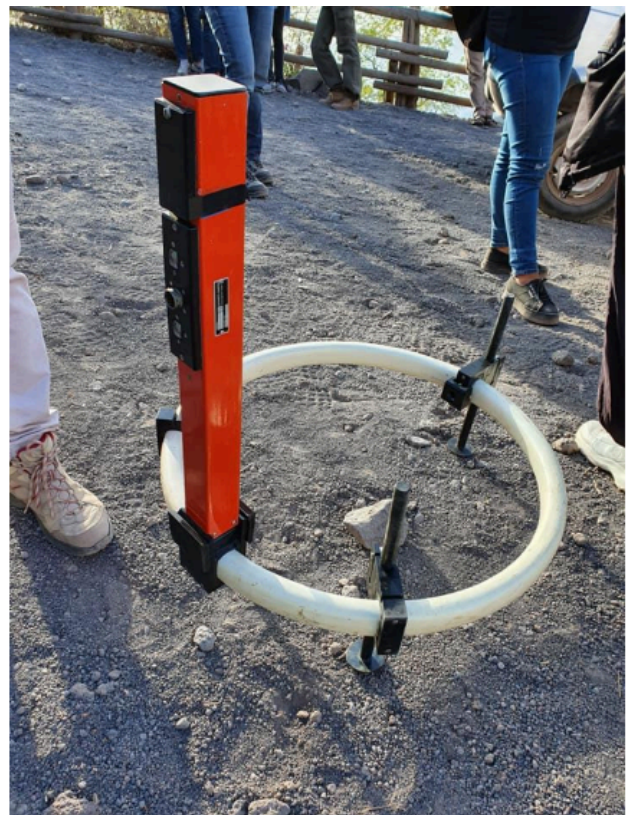
Figure 2 - The coil used by Menghini et al. to receive the electromagnetic response from the Earth. [8]
