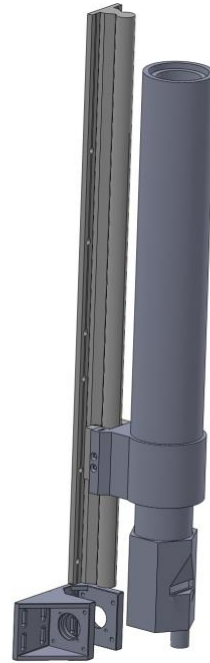
Figure 5: The rough sliding mechanism for the smaller tubes. Belt and idler pulley not shown
