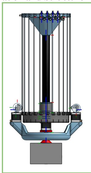
Harp core: made up of string base and harp hat, with strings. Carbon fiber PETG, core rod is a hollow tube of 1/16 wall steel.
