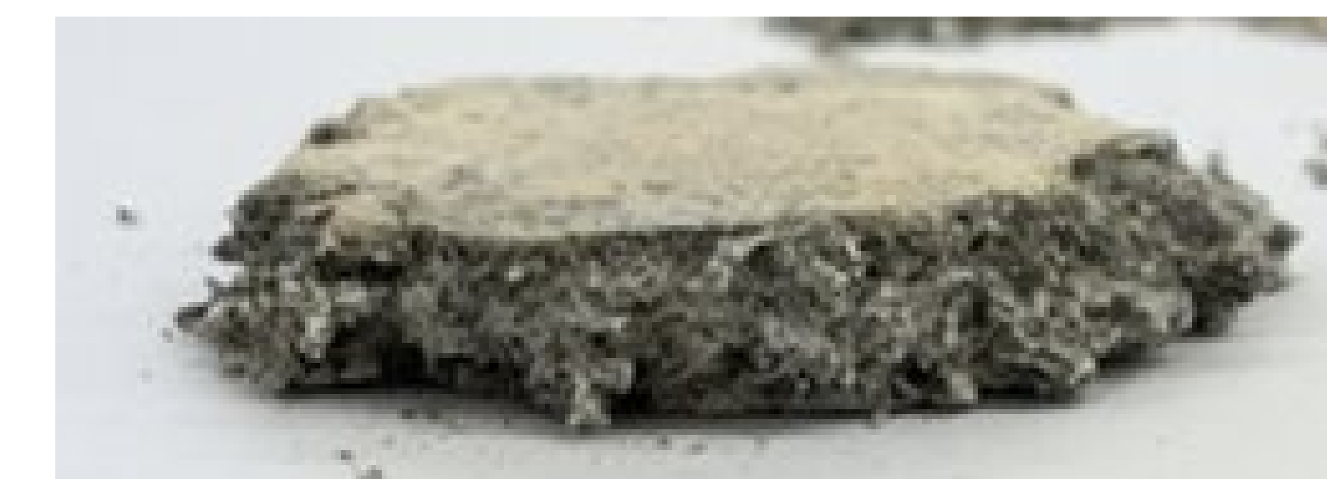
Fig 5. Image of compressed aluminum foam reinforced composite.
