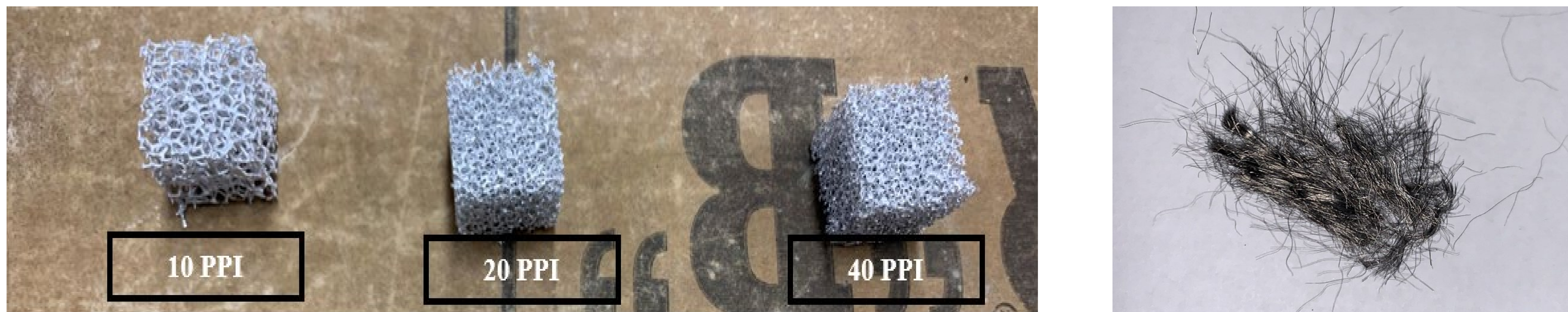
Fig 1. Images of the Duocel Aluminum 6061-T6 foams (left) and the Intramicron stainless steel A16 fibers (right).
