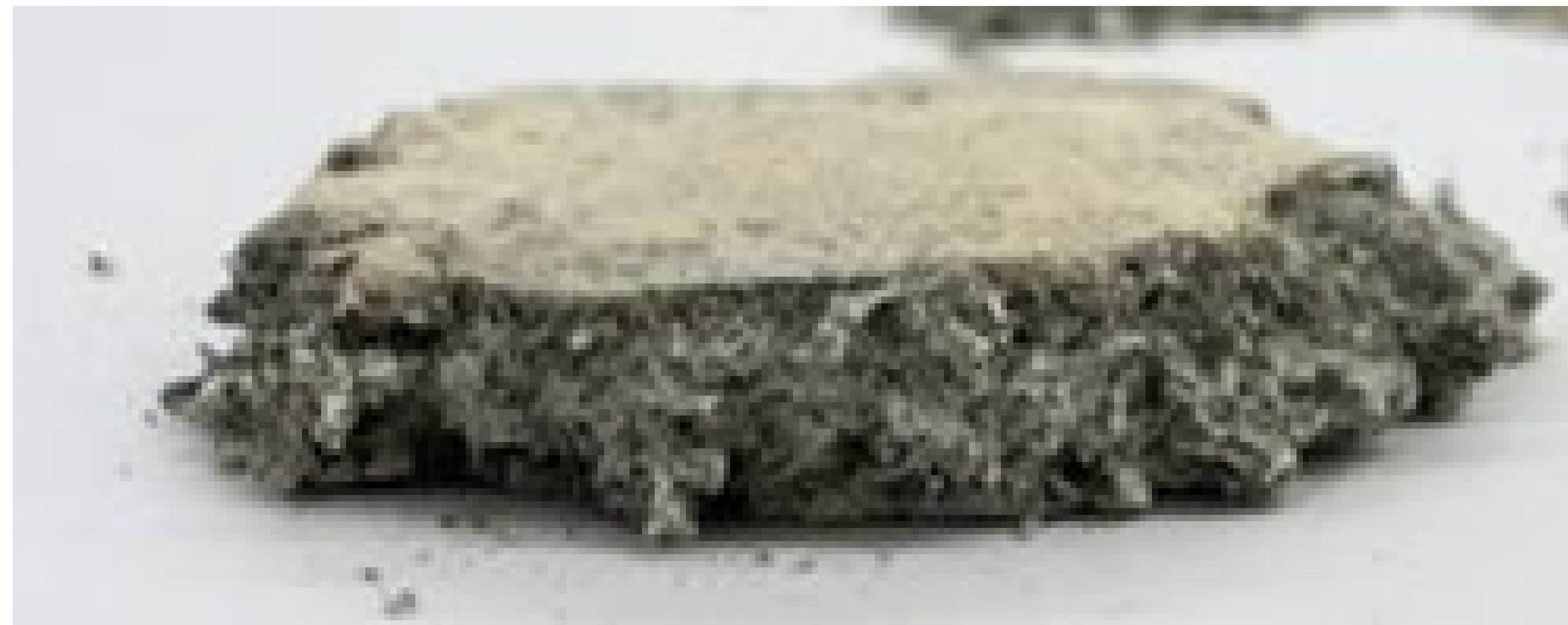
Fig 5. Image of compressed aluminum foam reinforced composite.
