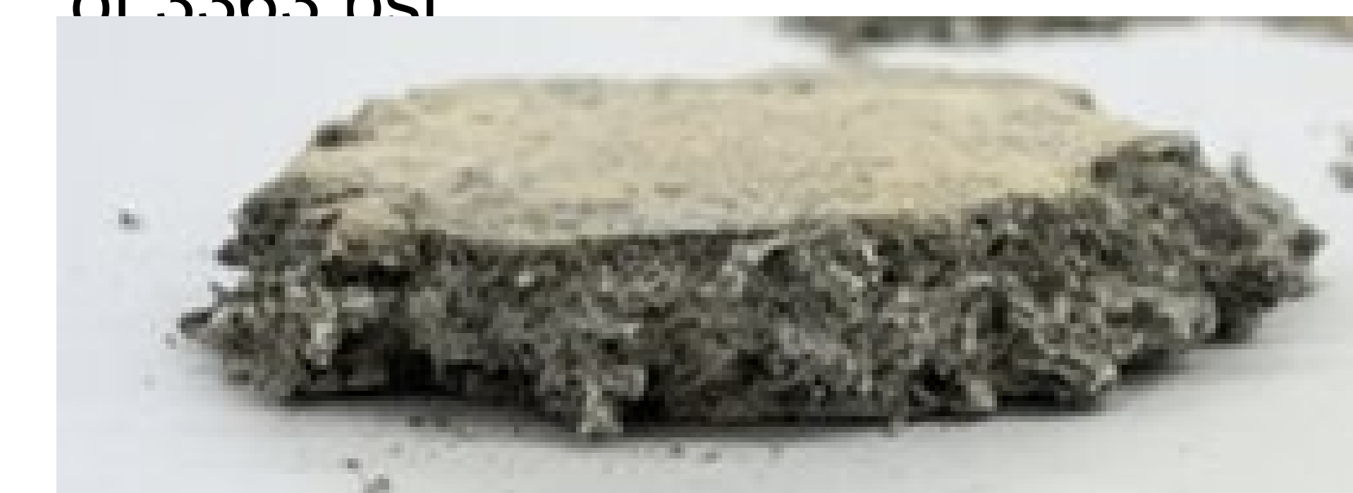
Fig 5. Image of compressed aluminum foam reinforced composite.
