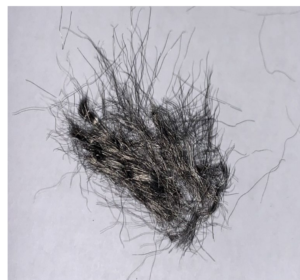
Fig 1. Images of the Duocel Aluminum 6061-T6 foams (top) and the Intramicron stainless steel A16 fibers (left).
