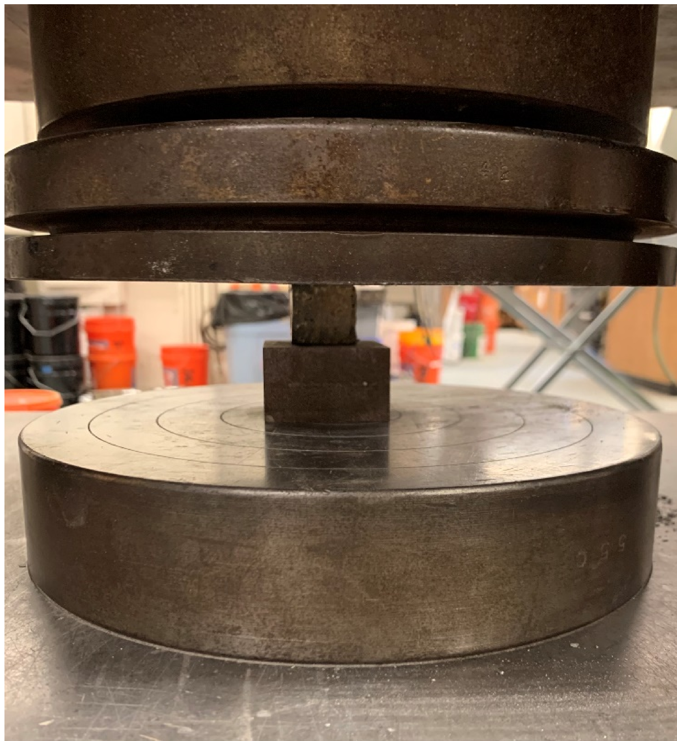
Fig 2. Image of an aluminum foam reinforced sample being tested in the Instron.
