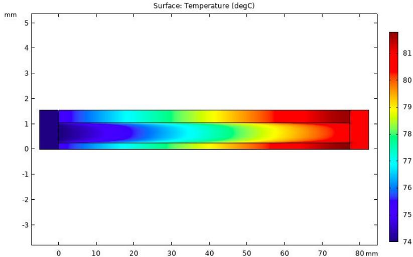
**2D temperature plot (°C) along a mid-channel slice with water (horizontal axis scaled 0.15)**
