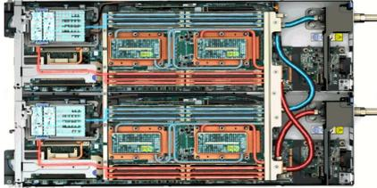
Liquid cooling with microchannel heat sinks
