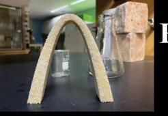
Engineered Biological Construction Material: Self-healing Carbon Negative Enzymatic Construction Materials (ECM)
