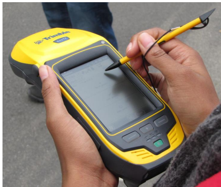
Figure 22: The GIS Trimble unit can record tree attributes and GIS coordinates of each tree (Project Team Photo).
