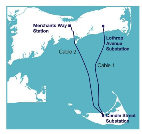
Figure 2: Nantucket's two undersea cables. (National Grid, n.d.)
