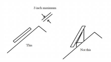
Figure 14: Diagram of solar panel orientation on a roof. (Historic District Commission, City of Methuen Massachusetts, 2016, p. 9)
