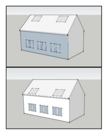
Figure 7: Guidelines encourage placement high on the roof (top) rather than near the eaves (bottom) (Way, 2009).
