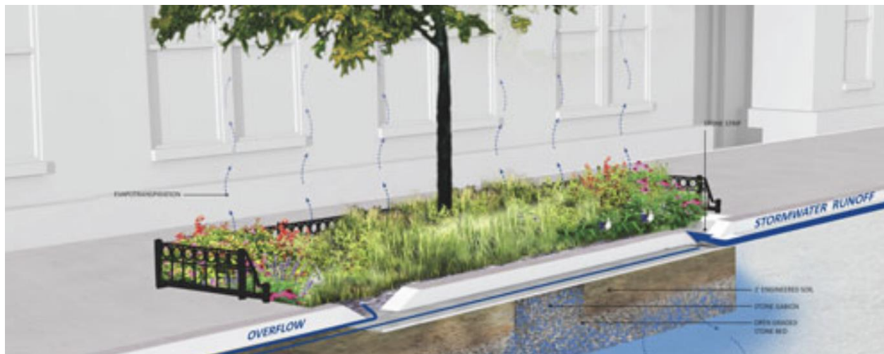
Figure 12: Illustration of rain garden on curb line (nyc.gov).
