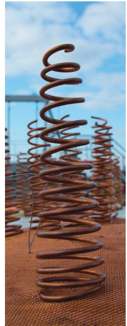
CONSISTING OF COPPER COILS ATTACHED TO A BLANKET MADE OF A LAYER OF COPPER WOOL SANDWICHED BETWEEN TWO LAYERS OF COPPER MESH, THE FLAME REFLUXER TRANSMITS HEAT FROM AN OIL FIRE TO THE OIL TO SUPERHEAT IT, INCREASING THE BURNING TEMPERATURE AND RATE, AND CUTTING EMISSIONS.
