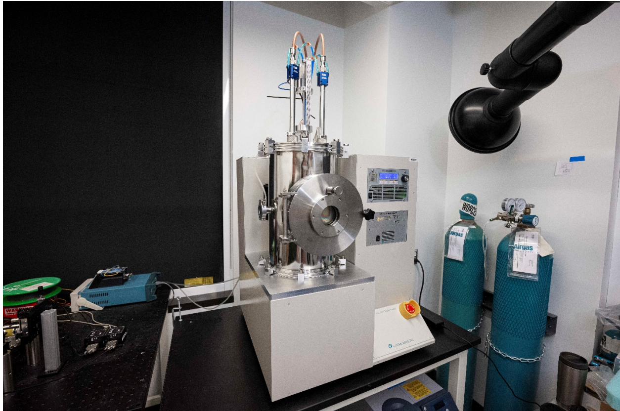
RF sputtering machine for thin ( <10 nm resolution) film deposition and fiber sensor functionalization
