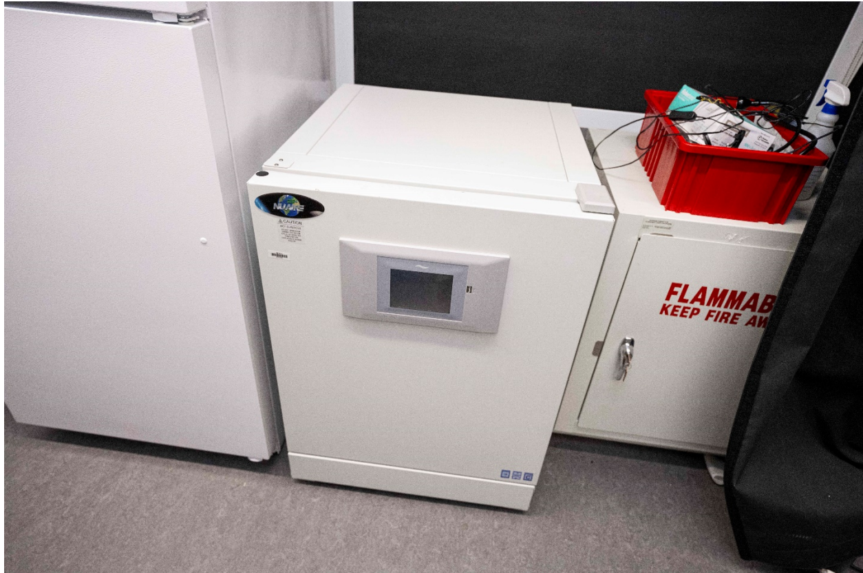
Cell incubator with environment (temperature, humidity, and gas) control.
