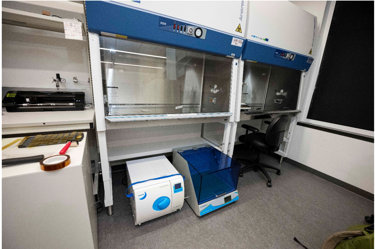
Microbiology equipment: biosafety cabinets, table-top autoclave, and bacteria shaking incubator
