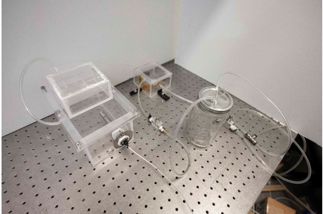
Custom gas chamber for humidity and gas sensor calibration and demonstration.
