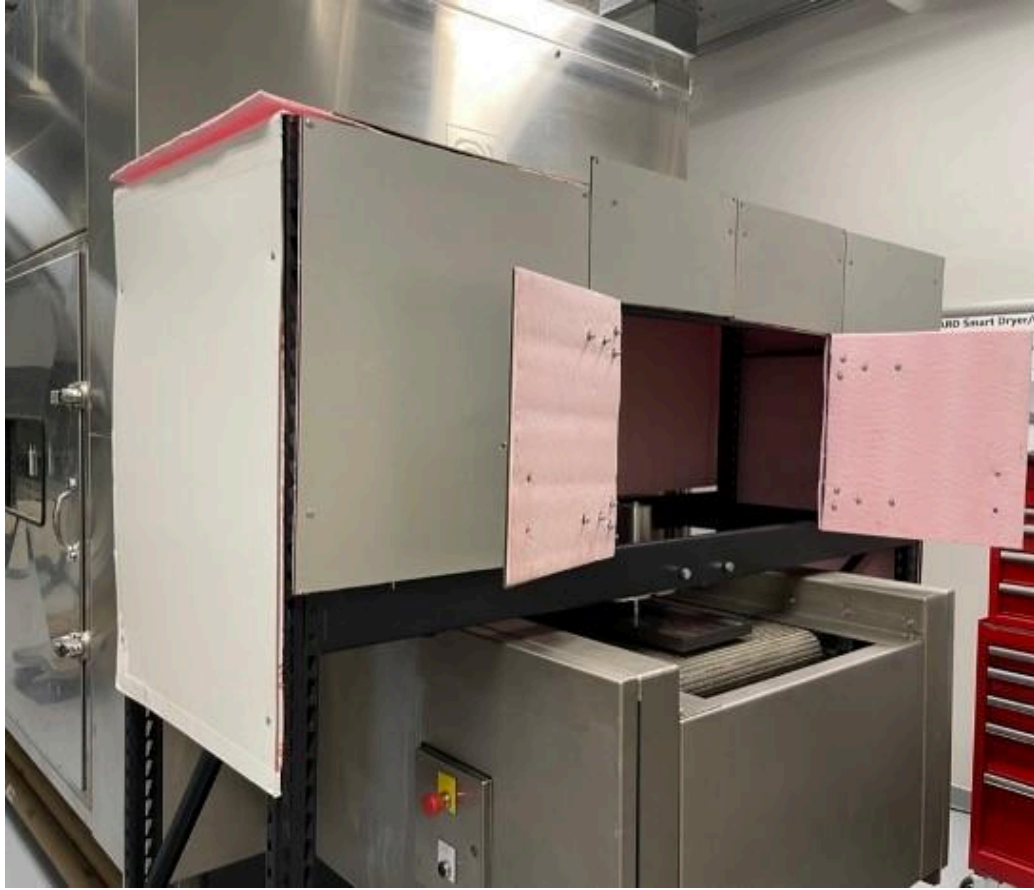
Airbone Ultrasound Transducer mounted at the entrance of the Smart Dryer
