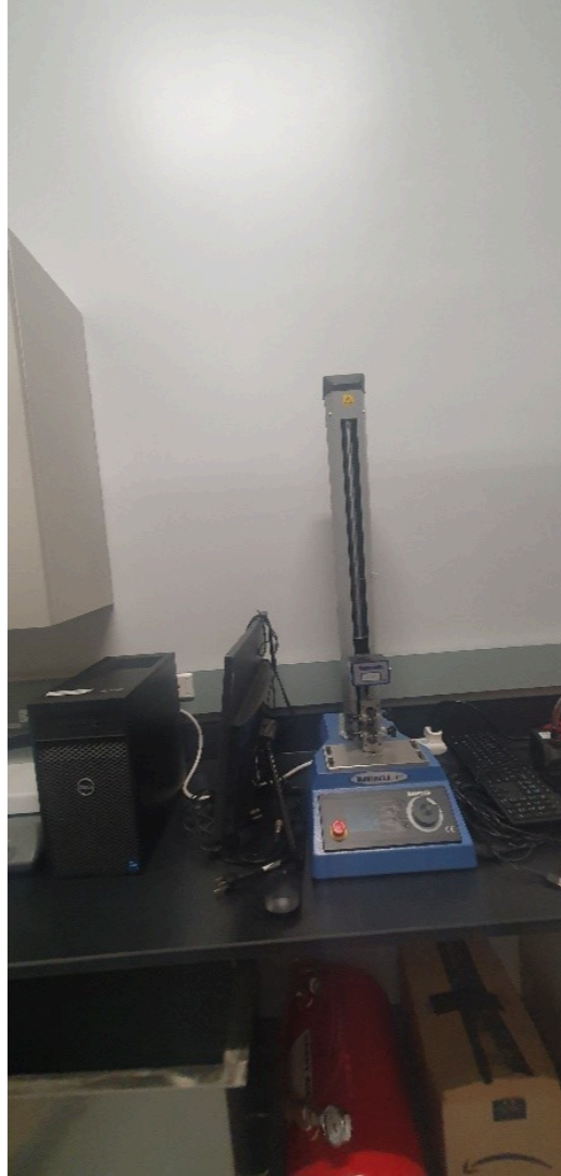
Mecmesin 2.5-dV. This tensile tester can apply tension and compression forces from as low as 2N up to 2.5kN to measure mechanical properties.
