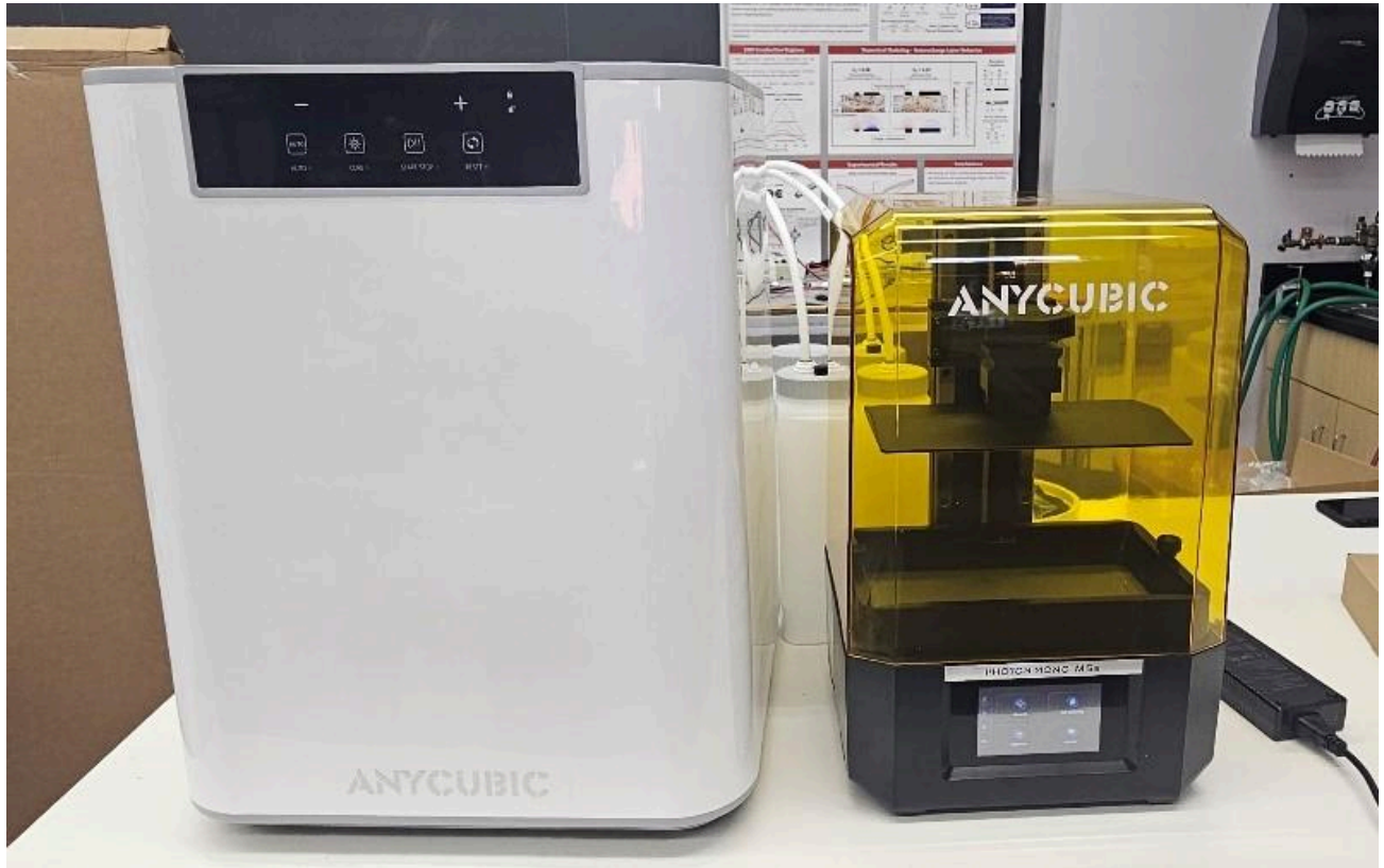
Anycubic Photon Mono M5s (3D printer) and Anycubic Wash & Cure Max (bath). The 3D printer is used to create resin structures for laboratory use.
