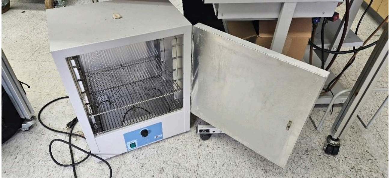
ThermoFisher Scientific Oven. This oven is used for small-scale heating and drying tests that don't require the smart dryer.
