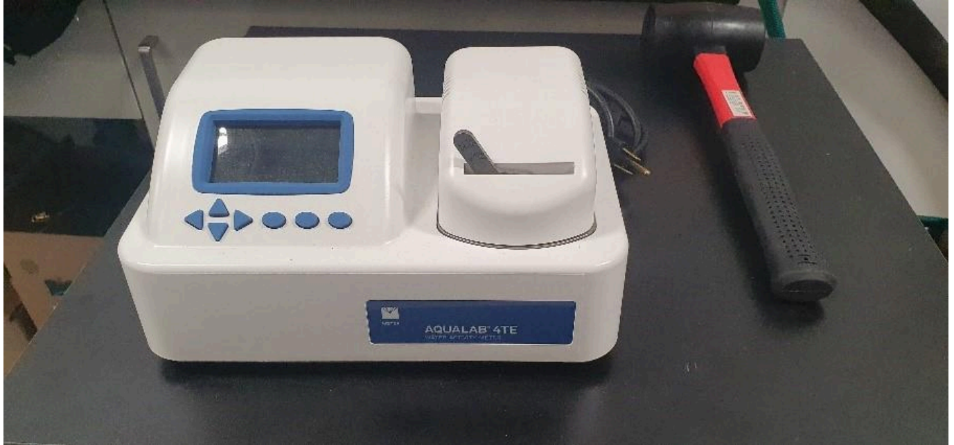
AQUALAB 4TE. This device measures water activity of samples to within 0.03. Especially helpful for food samples, water activity can be a good predictor of shelf-life.
