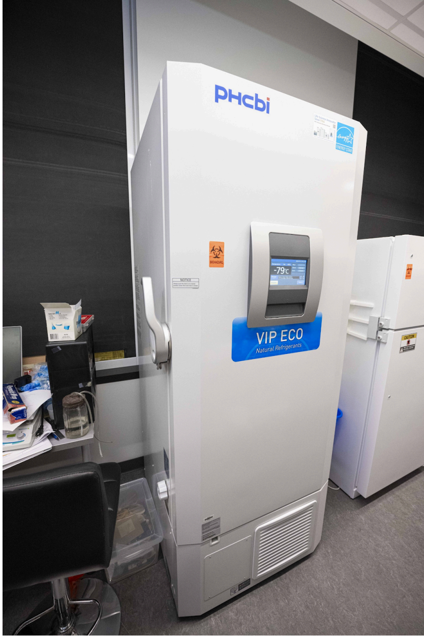
-80 oC freezer for biological sample storage
