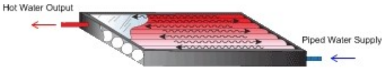
Integral SWH diagram with input from a public water supply, and output into household faucet.
