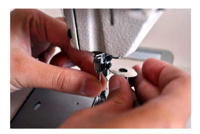
Insert the needle with the groove facing away from the machine. Tighten the screw until the needle is secure.
