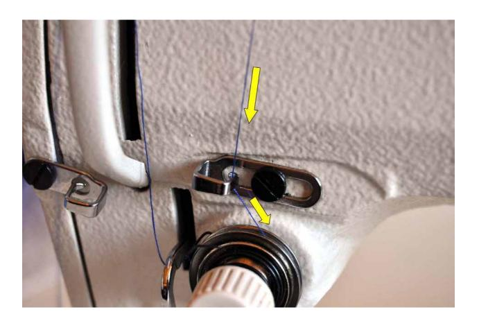
Run the thread underneath the circle and up through the small, dark metal piece on the opposite side.
