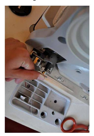
Run the thread underneath the circle and towards the bobbin.
