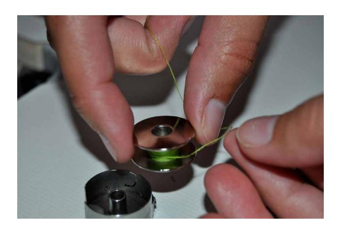
Add bobbin to bobbin case. Loop the thread under as shown below.
