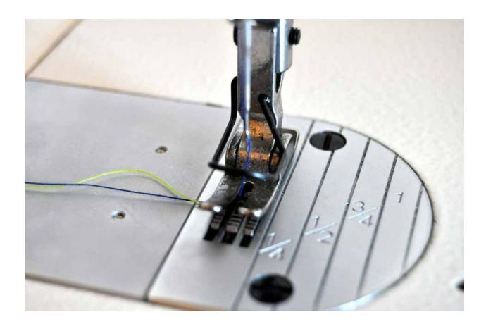
With the foot still raised, move a piece of fabric underneath. Release the knee lever.
