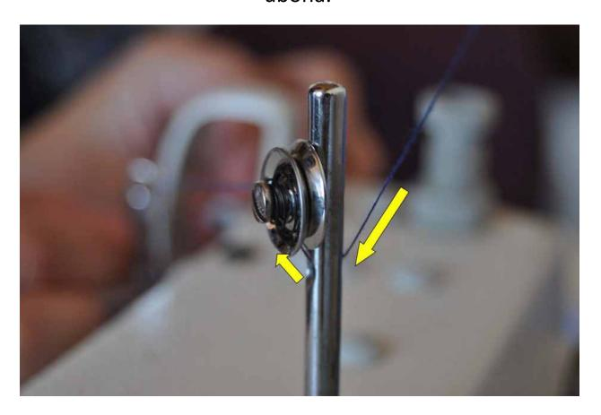
Once the thread is through the hole, place thread over the top of the circle.
