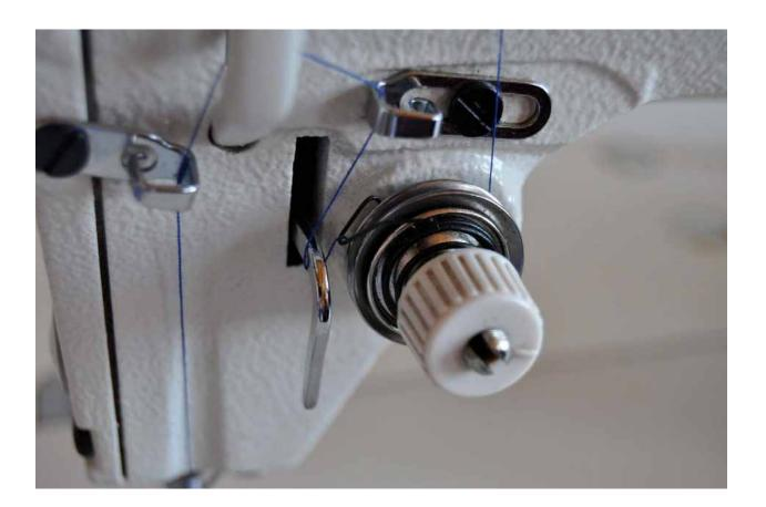
Run the thread underneath the larger L-shaped metal piece.
