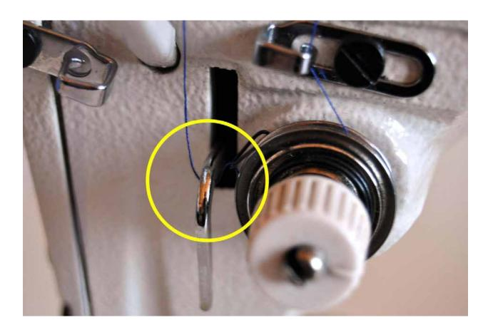
Run thread up and through the hole as shown below.
