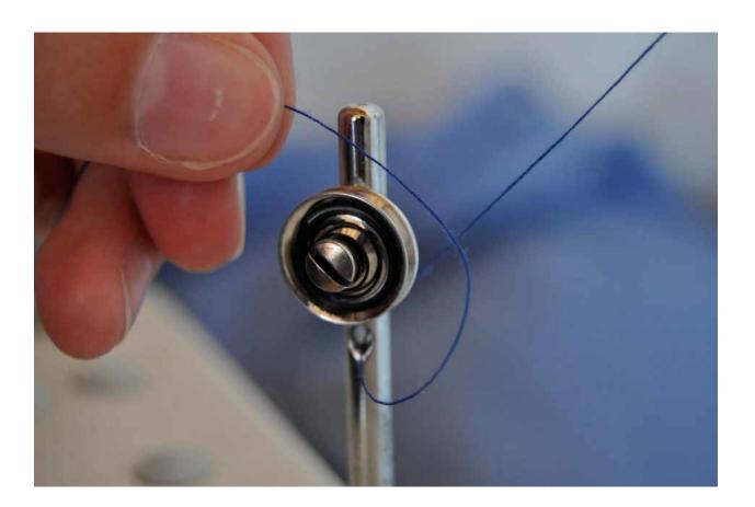
Pull thread down and slightly to the left. Pull the thread through the next section as shown in the images below.
