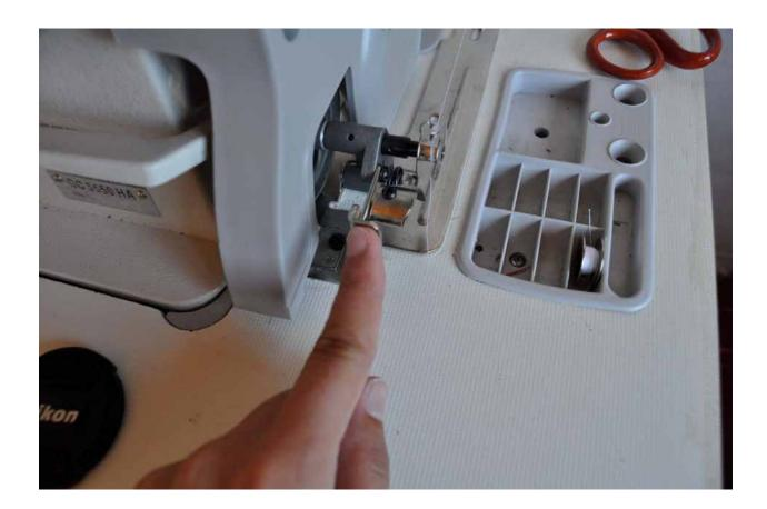
Press your foot on the pedal until the bobbin begins to wind. Remove your foot from the pedal when the bobbin is full.
