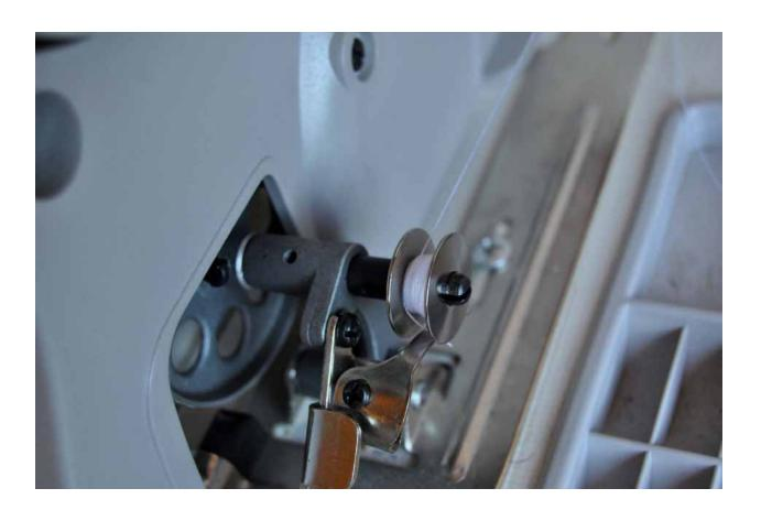
Remove the full bobbin from the side of the machine.
