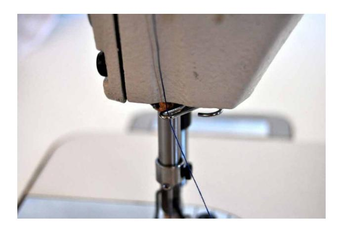
Pull thread through the hole from front to back as shown below.
