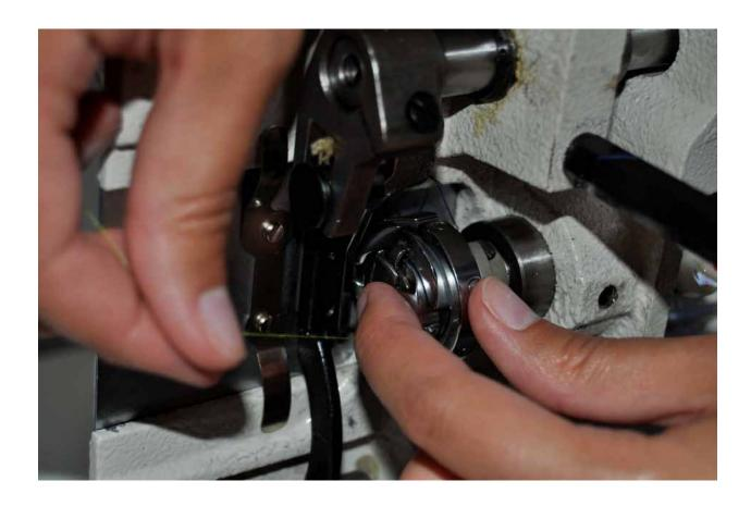
Lightly push on the foot pedal while simultaneously spinning the hand wheel and holding the main thread. The bobbin thread should catch within the first few wheel turns.
