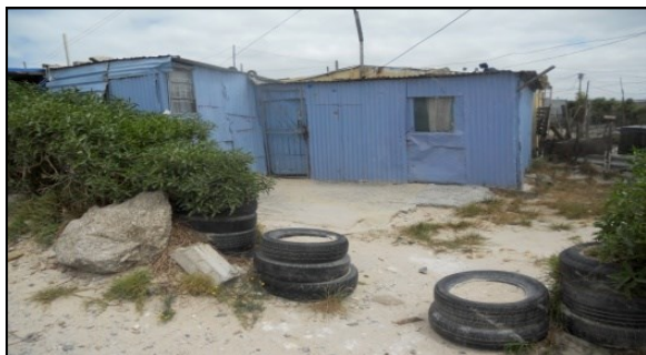
Figure 5: Stacked tyres filled with sand
